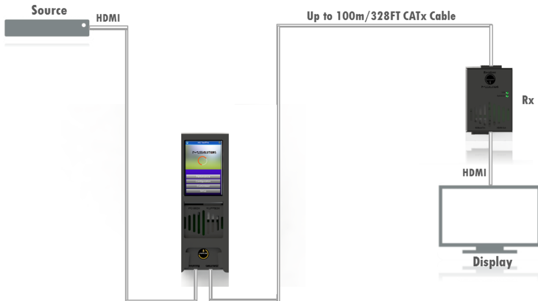
Figure 6: MS-TestPro Modules Test Setup
